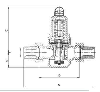
PRESSURE RATING PN25 TEMPERATURE RATING Max. 80°C MEDIUM Water Only CONNECTIONS Male tapered BS EN 10226-2 OUTLET PRESSURE RANGE 1-8 bar PRE-SET OUTLET PRESSURE 3 bar DESIGN STANDARD General conformity to BS EN 1567 APPROVALS: WRAS • PED 97/23/EC MESH SIZE: 1/2" - 1 1/4" - 0.60mm • 1 1/2" - 2" - 0.75mm
